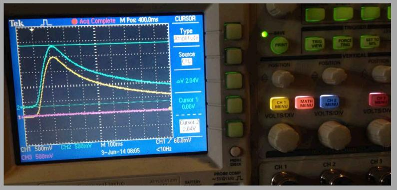
Determination of explosion pressure (reference pressure) Ex d I Mb Ex d lic Gb
