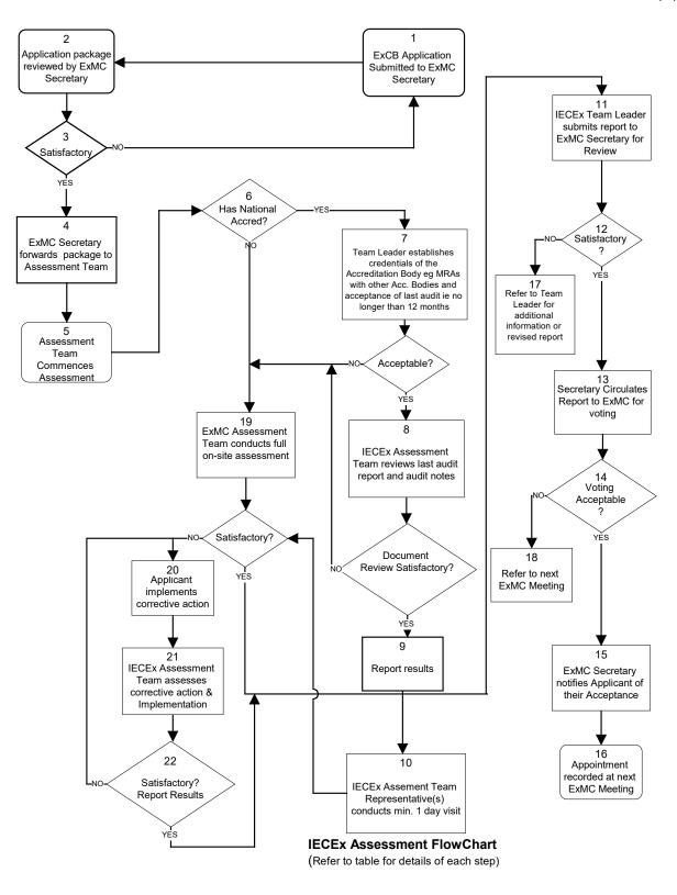
Figure 1 – IECEx Assessment Flowchart (refer to table for details of each step)
