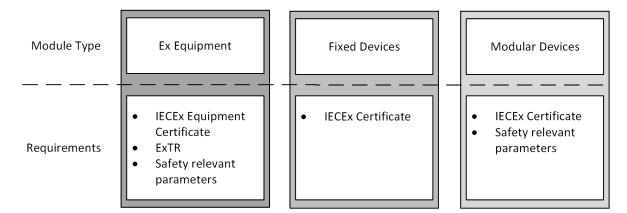
Figure 2 - Requirements of a Modular Combination
