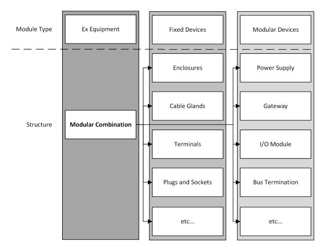
Figure 1 – Exemplary structure of a Modular Combination
